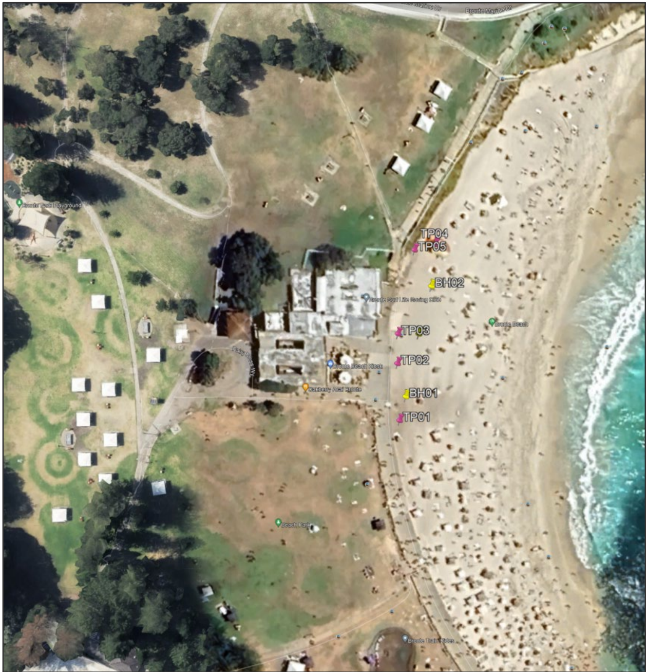
Figure 4-5 Testing locations for additional geotechnical investigation. BH03 is jointly located with TP03 (JK Geotechnics, 2024)
