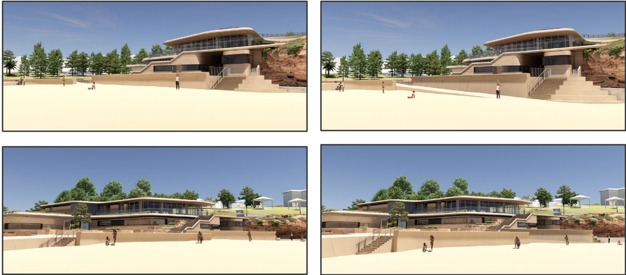
Figure 9-1 View analysis (Left) Reduced sand levels +3.00m AHD (Right) current sand levels +4.00m AHD. The recommend design scour level under present day climate conditions at the peak of design storm is +2.9m AHD (present day), reducing to +1.70m AHD (2050) and +0.35m AHD (2100) (refer to Section 5.2.3).
