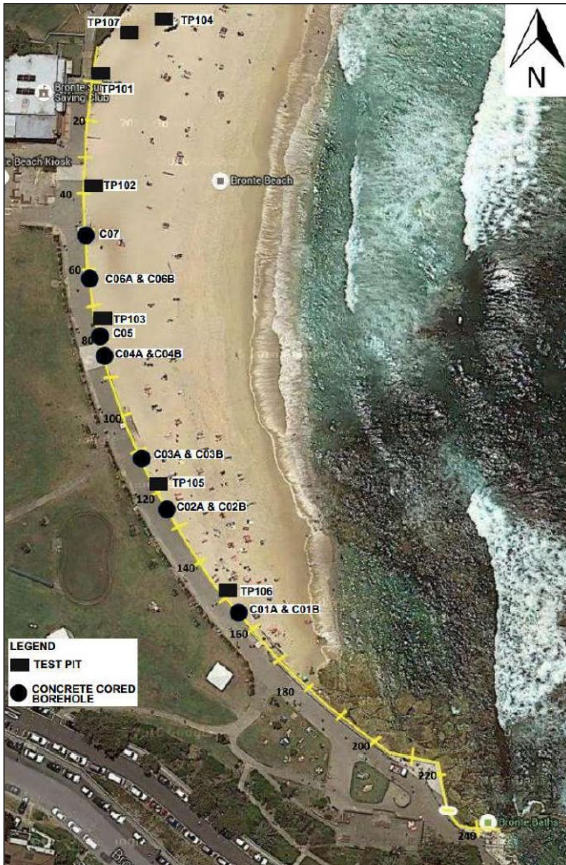
Figure 4-3 Seawall chainages and test pit and seawall coring locations (ARUP, 2016)
